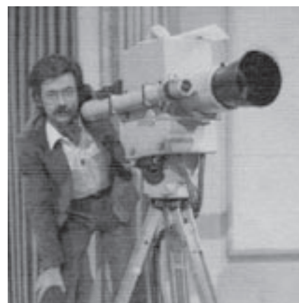
A Farnsworth type Image Dissector camera (plus a couple of Iconoscopes) was used at the 1936 Berlin Olympic Games. The picture shows the actual ID camera. Range finding was achieved by using a side-mounted optical scope. Video quality was reported as 'good'.
